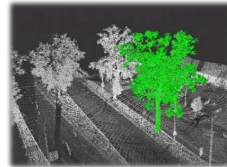
Terrestrial Laser Scanning
